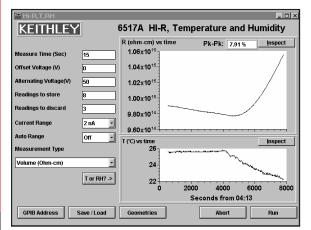
The Model 65 package can eliminate drift and noise in difficult materials, so it is possible to determine characteristics of the material that were previously obscured, such as temperature coefficient. The Model 6524 software allows graphing resistance/resistivity plus temperature or humidity vs. time on the same screen. This makes it easy to observe and calculate the dependence of a sample's resistance/resistivity vs. temperature and humidity.
